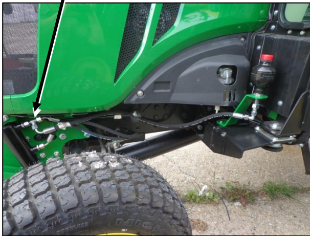
Fig. 39: Pressure accumulator – hydraulic system
