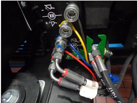
Fig. 12: Mounting the couplings of the front power system
