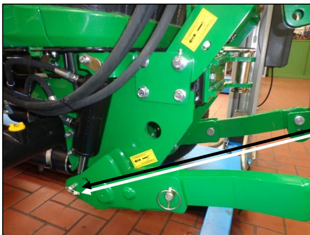
Fig. 46: Front power system lifted out
