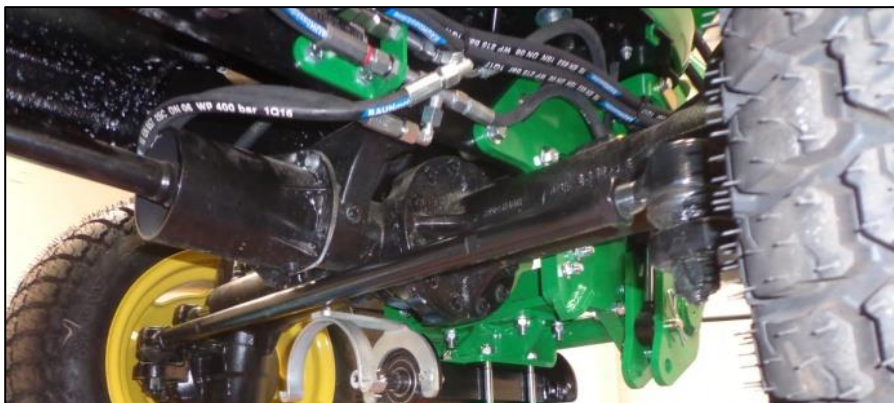
Fig. 10: Hose system left to right lift cylinder
