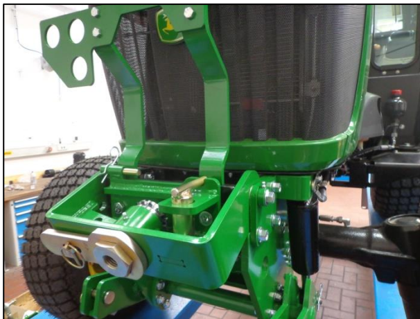
Fig. 5: Hitch, mounted with top link cat. 0 and hydraulic extension kit
