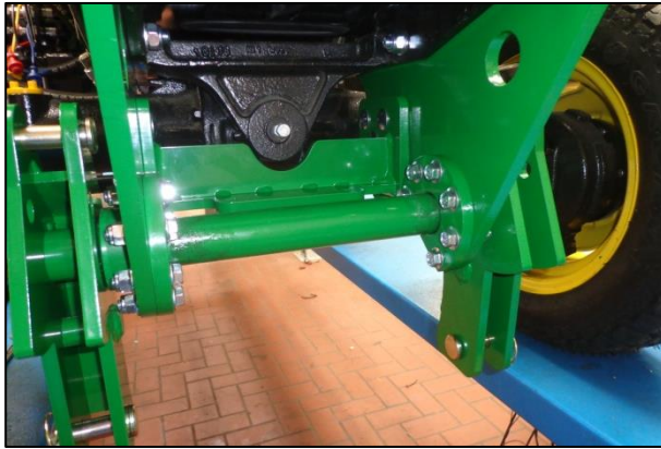
Fig. 4: Mounting of the lifting arm
