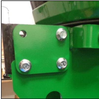
Fig. 16: Installing the side plate
