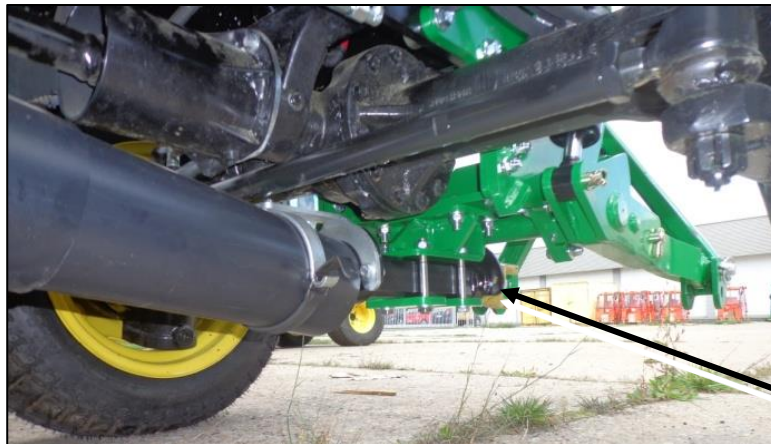
Fig. 34: Installation of the front PTO shaft on the front power system
