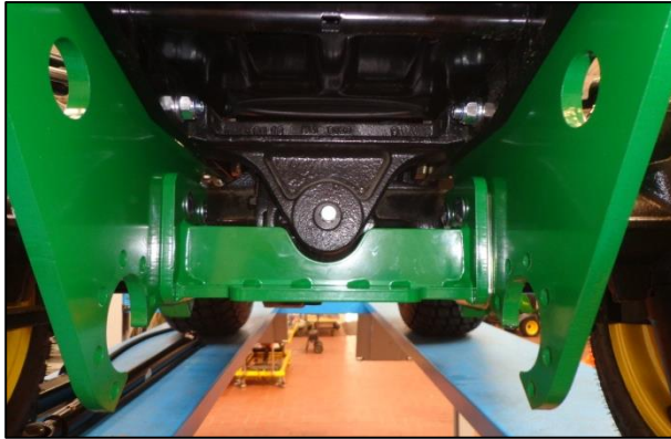
Fig. 3: Mounting the connecting piece
