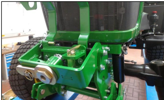
Fig. 18: Top link cat. 0 installed
