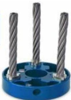
A robust weeding head with 3 quick lock replaceable wire brushes for use on professional petrol powered straight shaft brushcutters. When in use the wire cable unfurls and settles in a horizontal form to produce an effective surface brush.
