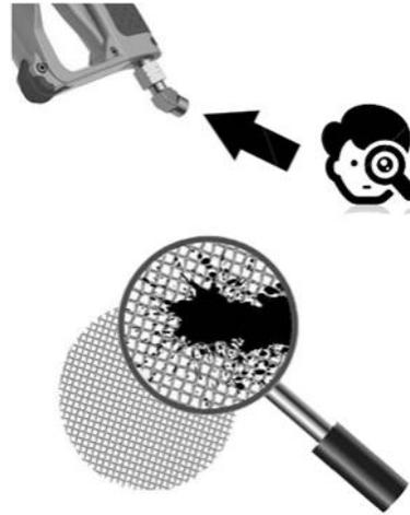
The rotating fitting is fitted with a mesh filter. This may become blocked by the pollution from a gas cylinder:
