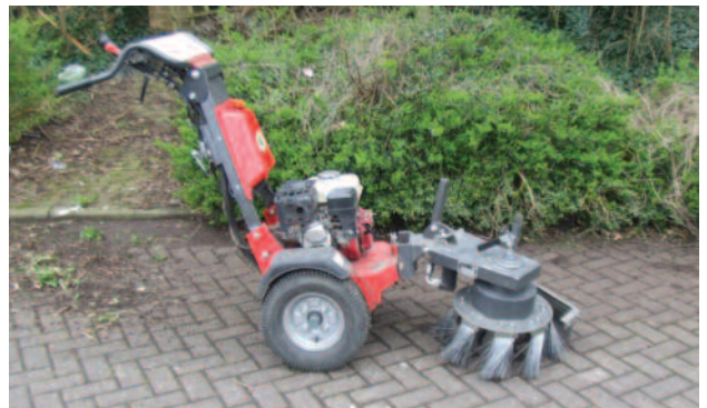
Brushing, an example of mechanical weed control
