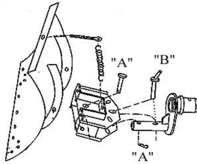
It may be necessary to loosen bolt A. Remove pin B, swing the snow plough in to the desired position and replace pin B. Retighten bolt A if required.
