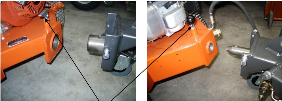
Pull locking Pin "A" then slide power unit and implement together
