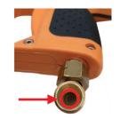
Clean (with a compressed air gun) the inside of the nozzle to remove all impurities (dust, grass, leaves, etc.)
