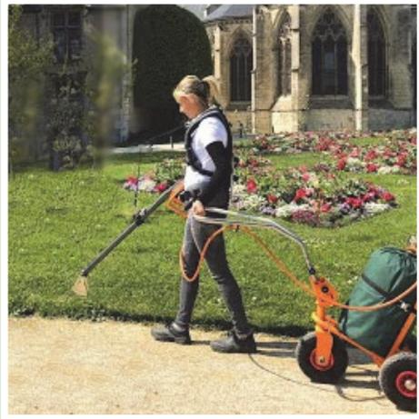
The thermal lance features an automatic ignition system when the gas trigger is squeezed and has an effective working width of 40cm. It may be mounted on the trolley in the centre or to the left or right allowing easy access to kerb edges. The nozzle may be rotated through 360° to tackle vegetation at different heights and angles
