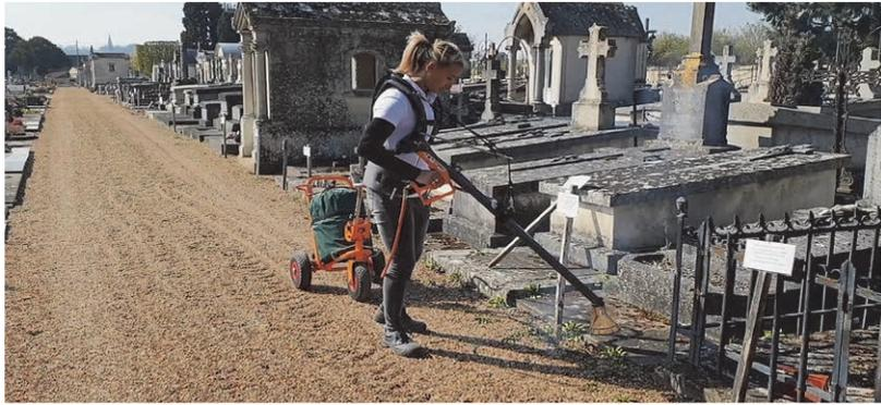
The Easy+ kit combines the mobile gas storage capacity with the Mini thermal lance mounted on the Ergonomic backpack allowing one hand to operate the lance and the other to position the trolley.
