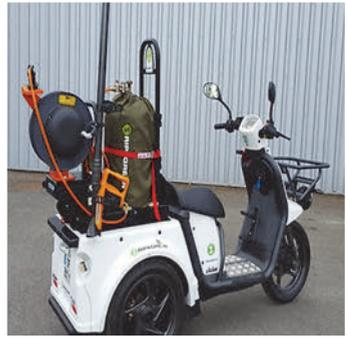
The Autonomy kit packs up quick and small to easily move from job to job with the mini thermal lance and automatic hose reel.
