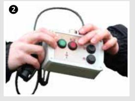
2 Electric remote control solenoid valves. Cab mounted
