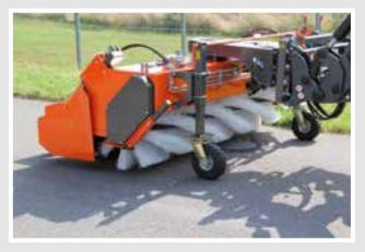
ABR 70 GS - Pallet tine pockets for forklift trucks and loaders with pallet forks
