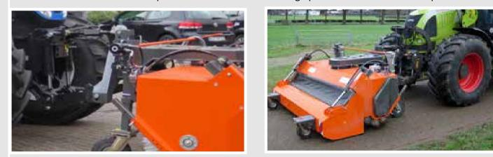
**ABR 70 Unimog** - Our special bracket and linkage system makes it possible to fit the sweeper to a Unimog or other vehicle 7500kg> with a DIN plate. Din plates are a standard fixed mounting system commonly found on highway vehicles of 7500kg>. The ABR 70 includes a powered lift and lower mechanism and therefore provides the ability to lift and lower the sweeper using a double acting hydraulic cylinder. The vehicle must be equipped with a suitable hydraulic service.
