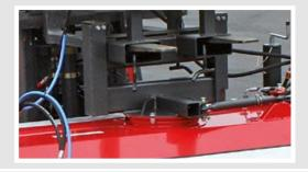
Vehicles with pallet tines can be connected to with this specially designed linkage from Kersten. A built in float mechanism allows the brush to cope with ground undulations without unsettling the tines. The top mounted linkage also allows manual angling of the sweeper, whilst keeping the sweeper close to the vehicle, making it much easier to manoeuvre.
