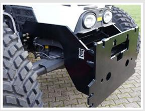
ABR 60 Tele DP - Multiple tractors? Our special bracket and connection system makes it possible to fit the sweeper to a Variety of linkage systems all from the same bracket. This allows it to fit to a tractor front loader, Telescopic loader, front loading shovel hitch and a Tractor 3 point linkage with CAT 1 or CAT 2 link arms.
