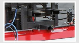
Vehicles with pallet tines can be connected to with this specially designed linkage from Kersten. A built in float mechanism allows the brush to cope with ground undulations without unsettling the tines. The top mounted linkage also allows manual angling of the sweeper, whilst keeping the sweeper close to the vehicle, making it much easier to manoeuvre.
