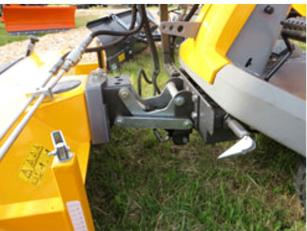
FKDR/HYD - The FKDR front linkage allows the fitting of powered and non-powered implements with hydraulic lift/lower and implement the angling from operators seat to a wide range of ride-on mowers.
