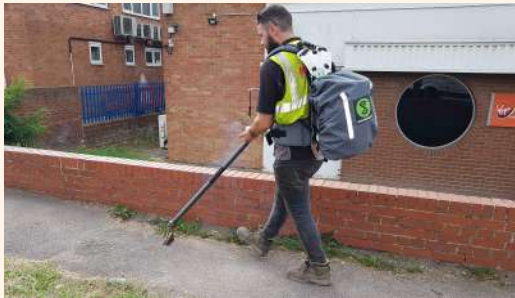
Examples of hot air weed control
