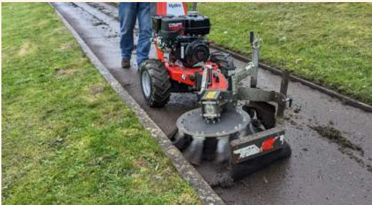
Examples of mechanical weed brushing
