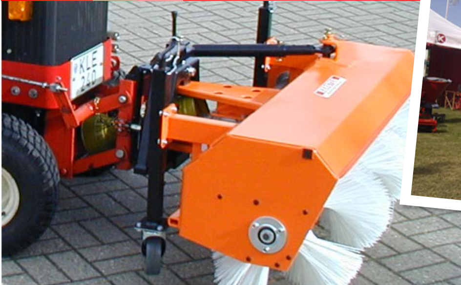
Hydraulic drive sweepers 125cm to 250cm working width with or without collection.
