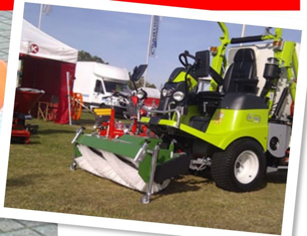
Hydraulic drive sweepers 125cm to 250cm working width with or without collection.
