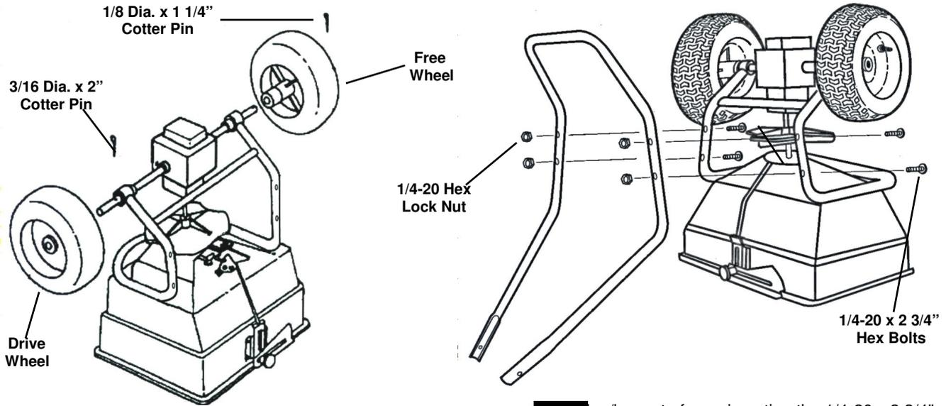
**1** Remove spreader and components from carton. Place spreader upside down. Slide drive and free wheels on axle as shown with the longer portion of wheel hub facing the frame. Secure free wheel with a 1/8 Dia. x 1 1/4" cotter pin. Secure drive wheel to axle with 3/16" Dia. x 2" cotter pin.
