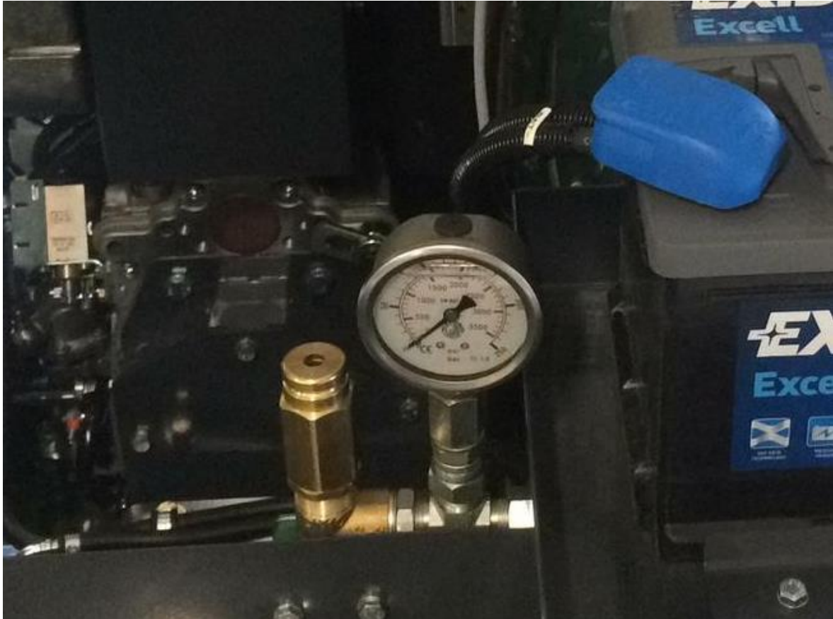
Picture 6. Safety valve and pressure gauge for ECO-mode
