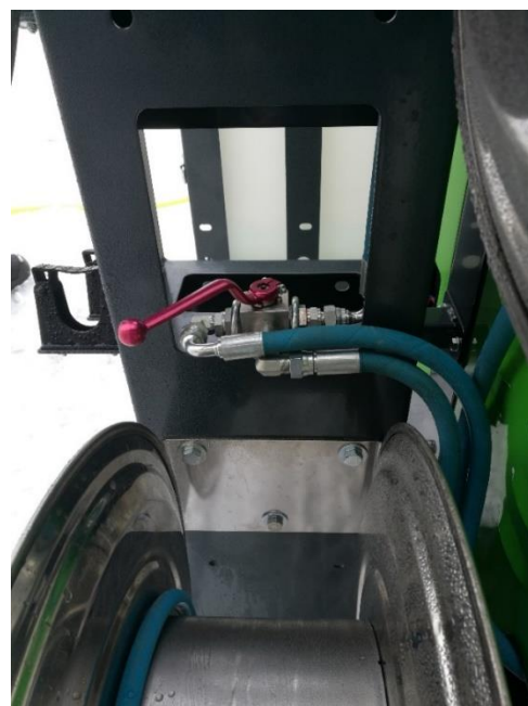
Picture 8.3. Water goes to both hose reels
