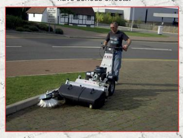
The Kersten Sweeper, with collector box and gulley brush fits the bill perfectly. It may be mounted on any of the Kersten K-Series Two Wheel Tractors From the 5.5hp K820 to the 9hp K2100 or, using the Kersten FKDR front linkage kit, it may be fitted to certain models of Ride-on Mower and tractor.
