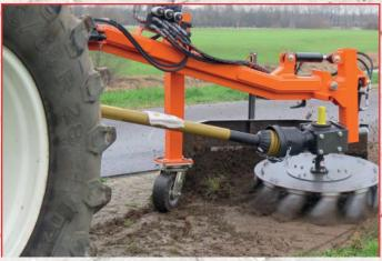
Frequency of use of the Weedbrush will obviously be variable, and perhaps seasonal. However, the speed at which moss appears in block paving means that on large sites it is almost inevitable that a surface will reach the condition where it needs a Weedbrush to rectify the situation, especially where trees and hedges are present. Our best advice however, is that prevention is better than cure.
