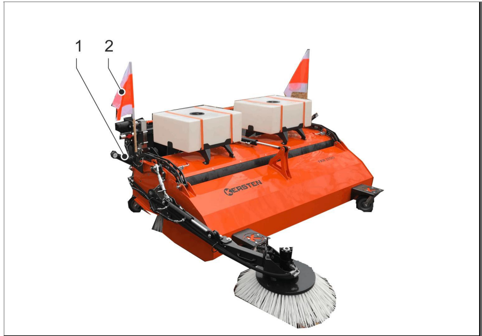
Fig. 16: Front sweeper with warning flags and marker lights
