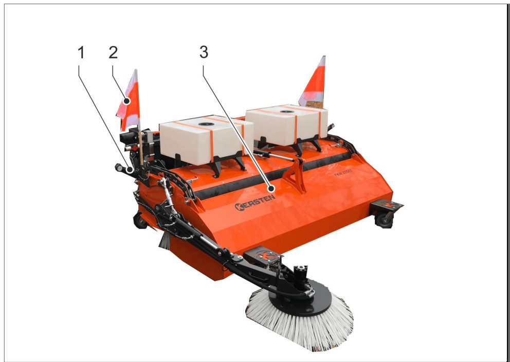
Fig. 5: Splash guard with signal band 1 marker lights (optional) 2 warning flags 3 dirt collection
