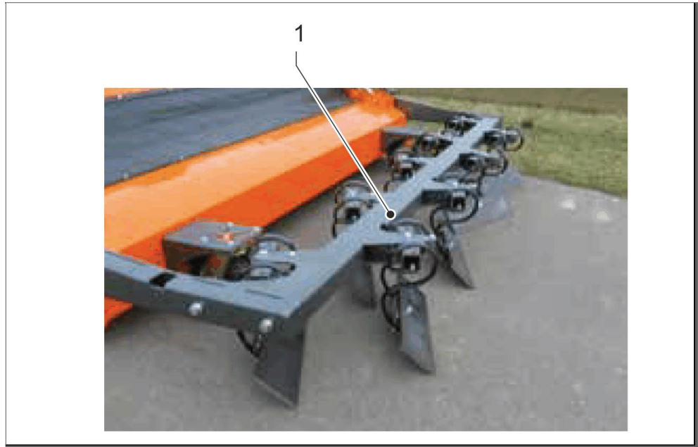
Fig. 13: On scratch bar (collecting operation)
