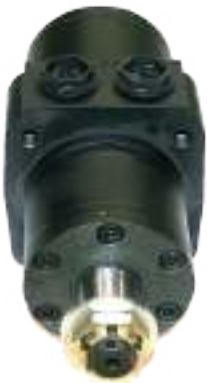
Individual steering motor for both wheels
