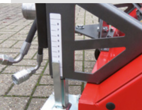
Stepless height adjustment of the sweeping roller
