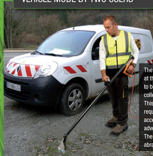
The driver positions their vehicle at the centre of the various areas to be treated while their colleague weeds using the lance. This arrangement deals with the requirement to quickly treat large accessible but scattered areas of adventitious plants. The gas pipe is treated against abrasion.
