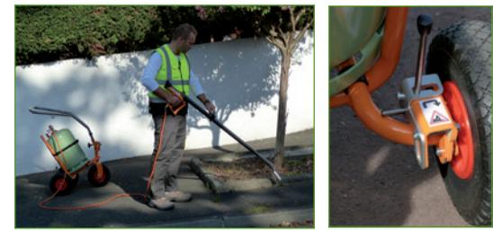
A parking brake allows the trolley to be stabilised when operating on a slope.
