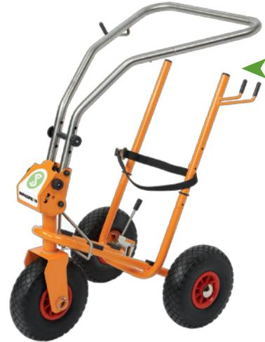
The Ripagreen® frame is built using rugged and durable materials; epoxy-painted steel tube for the supporting frame, anti-corrosion treated steel wire and tube for the control tiller and equipment such as the brake and the nozzle orientation device. However, it weighs only 12.5 kg and folds down in a few seconds to optimise storage.
